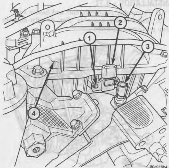
**Fig. 8 MAP SENSOR / ECT SENSOR - 3.7L V-6**
