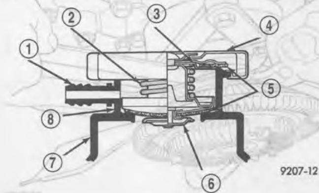
**Fig. 29 Radiator Pressure Cap Filler Neck**
