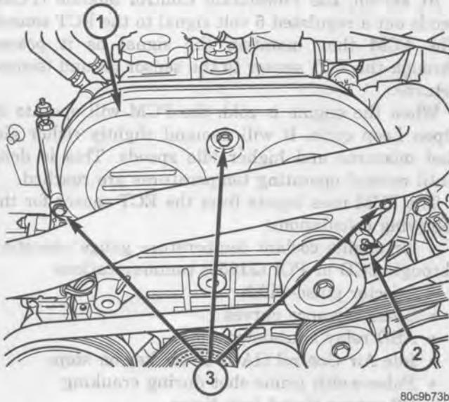
**Fig. 7 ECT AND UPPER TIMING BELT COVER/
