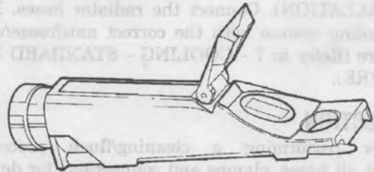
**Coolant Refractometer 8286**
