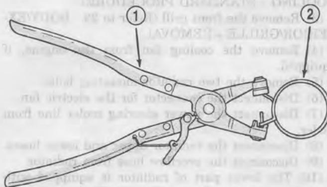
**Fig. 18 Hose Clamp Tool - Typical**
