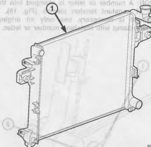
**Fig. 17 Cross Flow Radiator - Typical**
