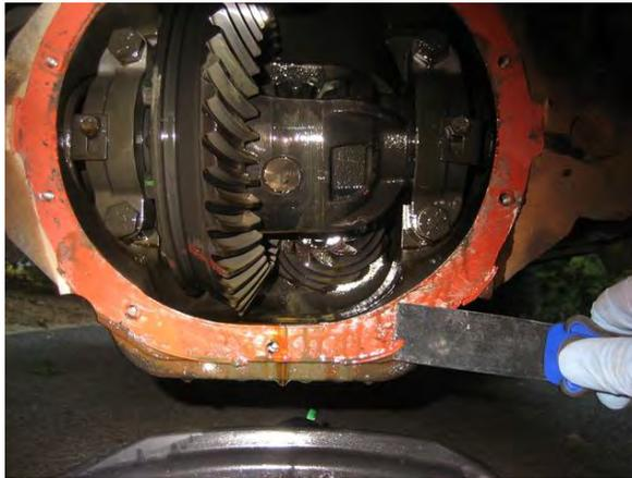
Got the scrapper out to remove the old RTV from the housing.
