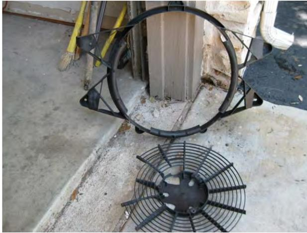
Notice the lug on the Hayden fan has been cut down to where about 1/8 of the bolt hole in the lug is left.
