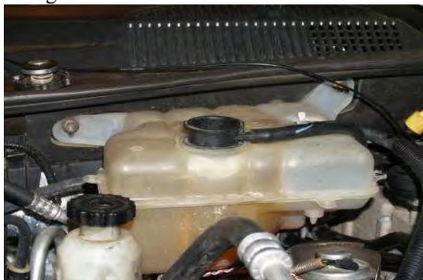
7. Disconnect the three rubber coolant lines attached to the bottle with constant tension clamps. Then pull
