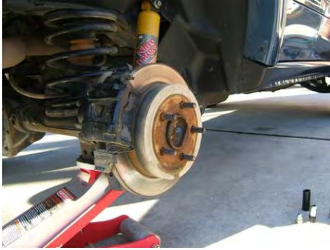
Make sure the rotor turns easily to begin with.. Take this little plug out to get to the star wheel:
