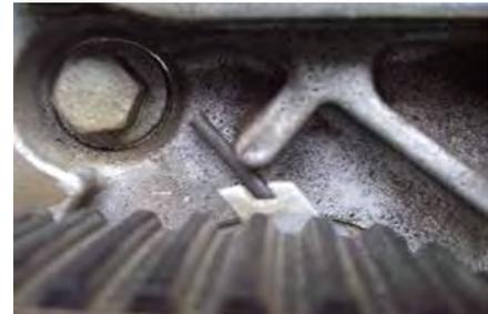
16. **Remove the two camshaft pins; flywheel pin; and cam gear holder** and rotate the engine **clockwise** 720 degrees (2 revolutions - may need to do 3 to get witness marks to align); verify that the timing belt tensioner is still in the proper orientation per the right hand picture above. Readjust tensioner as necessary **and** double check that the cam pins (ideally flywheel pin also) can be reinserted. **Be sure to double check all pins are removed.**
