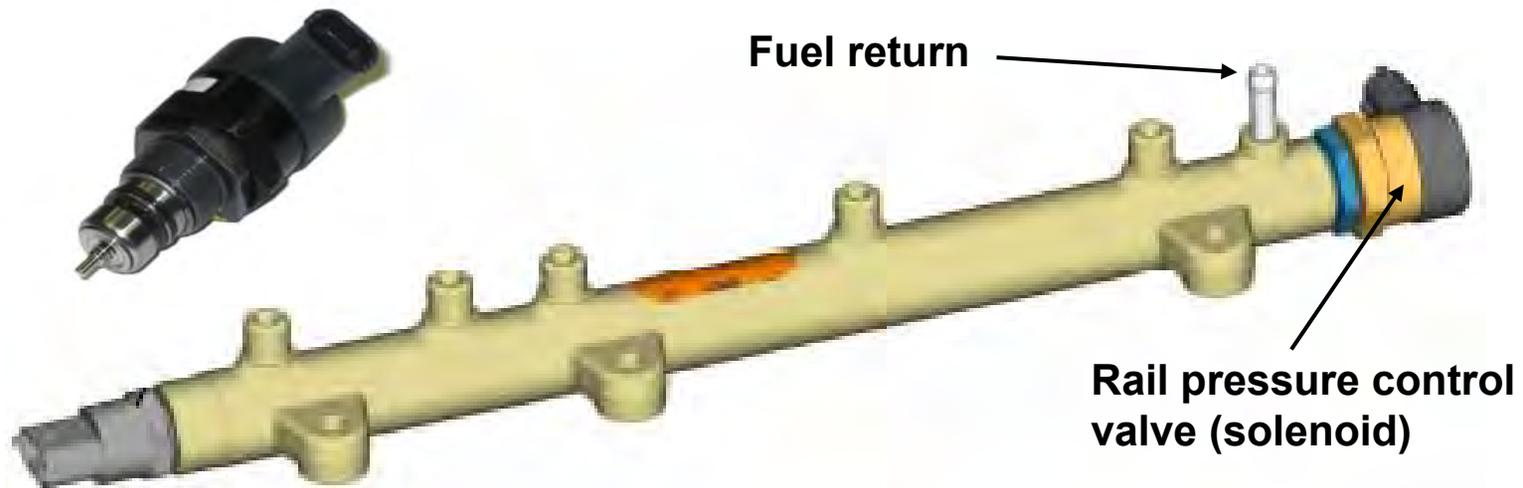
The valve controls fuel pressure by opening and closing a return port in the rail.
