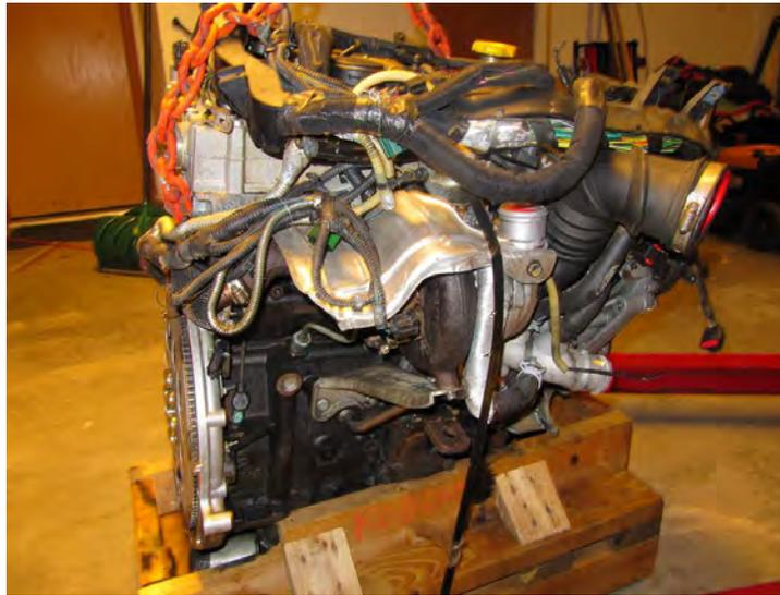
Passenger side view showing rear unused oil port (this can be used to mount an oil pressure sensor in the upper engine pressurized oil gallery "before" the turbo oil feed), turbo supply line and on the left rear the crank position sensor with heat shield removed for access
