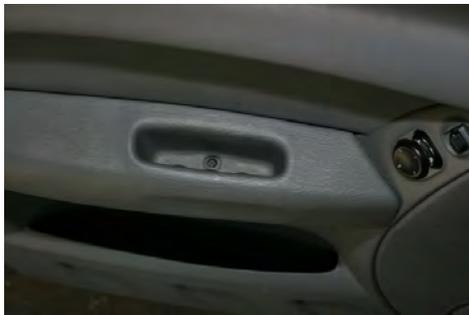
Other than these two screws, the door panel is only attached by 11 plastic body panel fasteners along the outer perimeter of the door. You simply need to yank on the door panel to get it free from these. I used a putty knife along the bottom of the door to pull the panel far enough away from the door so I could get my fingers in so I could give it a good tug. Once free of the plastic paneling pins, you lift the entire panel upward to get it free of the window and lock.
