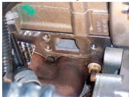
Remove 3 10mm bolts securing the thermostat to the block. All 3 can be reached with a 2.5 inch socket extension on a 6 inch wobble end socket extension. Remove the thermostat, scrape the gasket material off of the engine block and clean with acetone.
