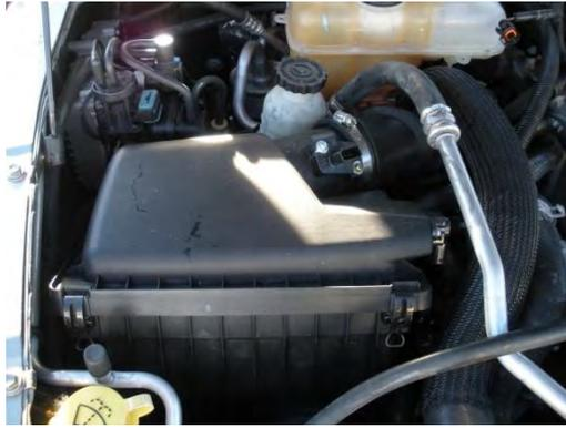
If the grommet comes out put it back into the fender it makes it easier to put the air box back later.
