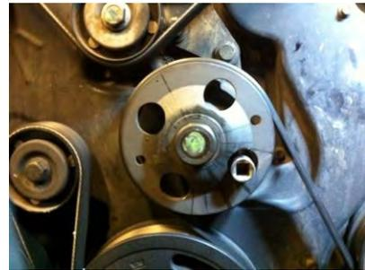
4. Relax serpentine belt tensioner (15mm bolt) by rotating clockwise and remove accessory drive belt.
