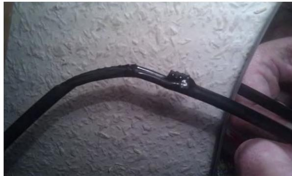
here are some aditional pics of the Line. it is the one with slightly larger diameter, which is connected to the solenoid by downward U flexible tube. the point were it is melted is indicated by the knife: on that pic the 2 lines from the solenoid are still taped together, the protectors are removed. the one damaged is the larger and shorter line with the downward U at one end
