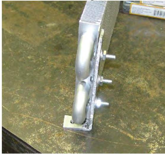
An easily fabricated aluminum L-bracket.
