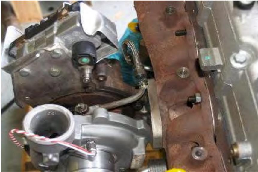
31. Slide the gasket on the studs at the rear of turbo for downpipe.
