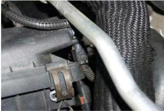
5. Remove clean air duct from turbo compressor using 8mm socket and extension. Remove CCV breather hose at the CCV on top of engine. Set to the side.
