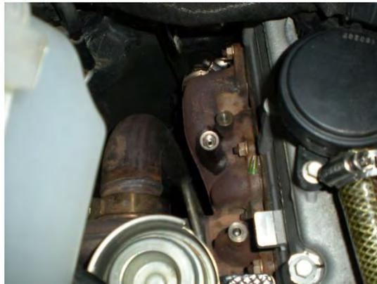
Cut the exhaust heat shield to allow the probe to pass through:
