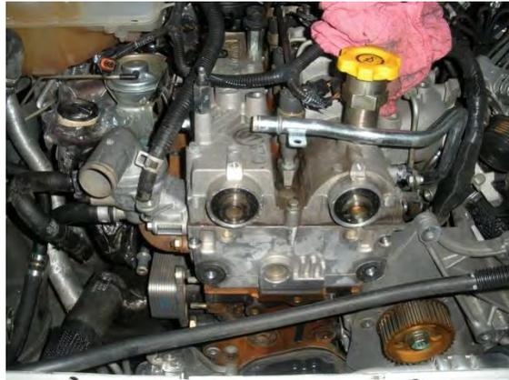
Install the back cover and the cam sprockets leave them loose then the idler pulleys and the tensioner then the timing belt. Not all torque wrenches work backwards keep this in mind when you put on the idler pulleys.
