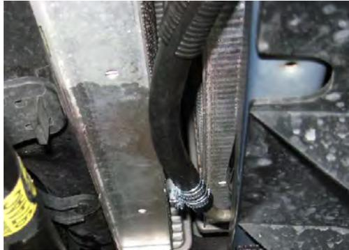
This is the line to the new cooler. I double-clamped it since the hard line isn't flared.
