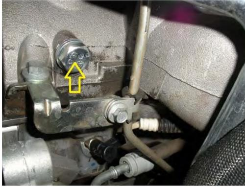
VM.1053 is just behind the thermostat housing about in the middle of the valve cover. After getting the cam locking pins in with the fuel pump either lined up or marked you will need to jack **(NOTE - no need to do this for just timing belt job)** the jeep up enough to get under it USING JACK STANDS not just the jack.
