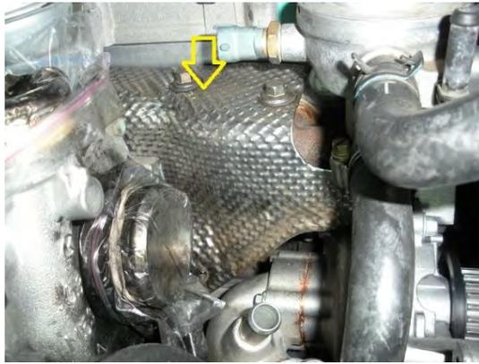
After all the coolant is drained (**NOTE - no need to do this for just timing belt job**) from the hoses you can remove the outer timing belt cover.
