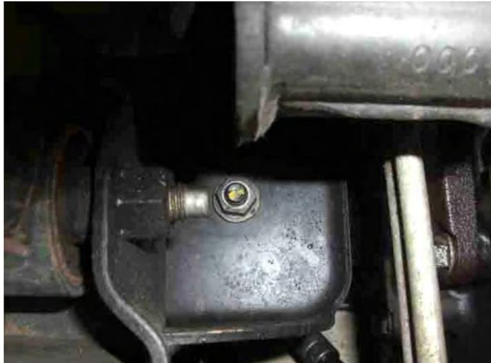
7. Use a jack with a short 2x4 wood piece and locate it on the oil sump toward the passenger side. Lift the engine as high as it will go making sure the jack is not catching on the axle or cross member.
