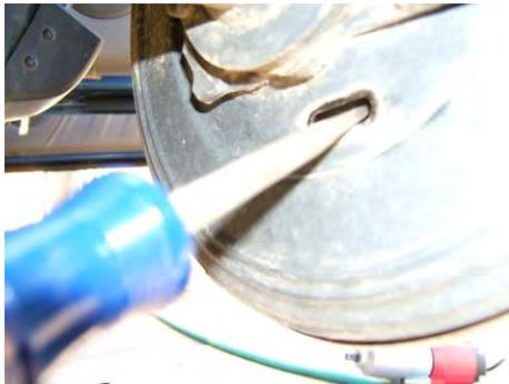
Release the handle and check for drag.. Put the plug back in and put the wheel back on. Again, check for drag by turning the wheel.. There should be some drag which is normal.. Just not enough to stop the wheel as soon as you stop turning it.. repeat on the other side.. Be sure to click the Ebrake handle again 3 clicks for the other side..
