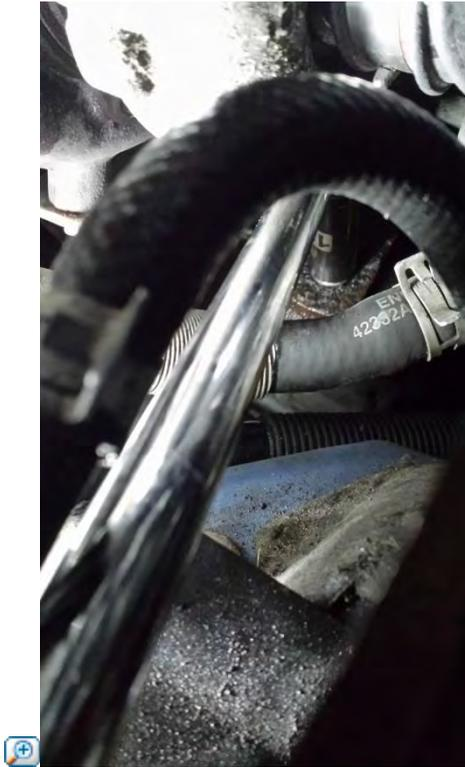
I'd like to highlight the importance of properly seating the socket on the nut, especially when using a flex joint it may not be so easy right away, maybe the nut is dirty, or maybe just a bad day, take your time and properly seat the socket on the nut, so it will untie nice and easy, without rounding the edges. Especially with this cramped space in this car's under the hood, rounding the edges of the nut can result in few more days of work.
