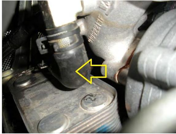
Well it's all apart now and you just have to put it back together. So reinstall the water pump only connect the bottom hose.
