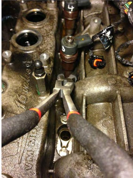
For the injector number 1, you can use a socket under the plier for a better angle. Once injectors are gone, proceed in removing the bolts from valve cover. You can reuse them at installation, but I'd recommend buying at least 2 long ones (id parts has them) since if you cut the bolt hex head, file that end a little, you can use them when installing back the valve cover:
