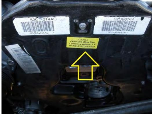
Find and remove the plugs in the valve cover. I had to use vice grips to break them loose the Allen wrench was stripping out.
