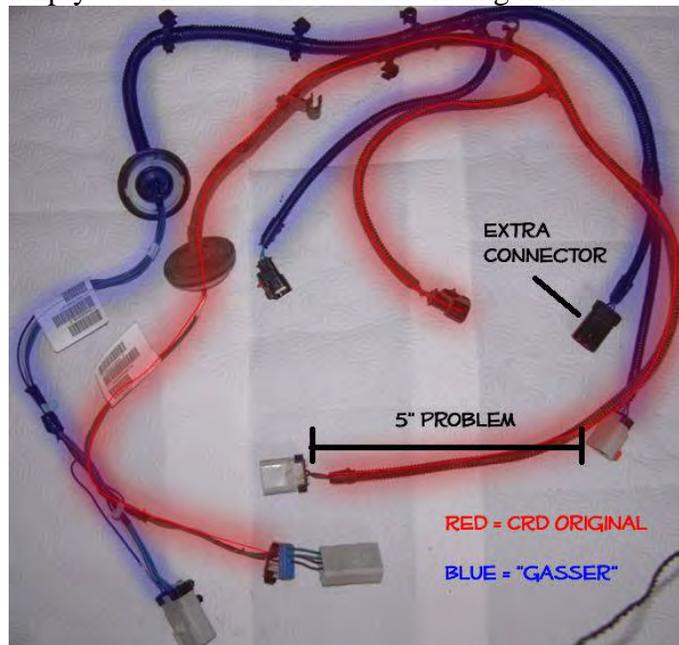
This involves partial disassembly of the harness by removing the hangers and untaping the loom. Below illustrates two things.
