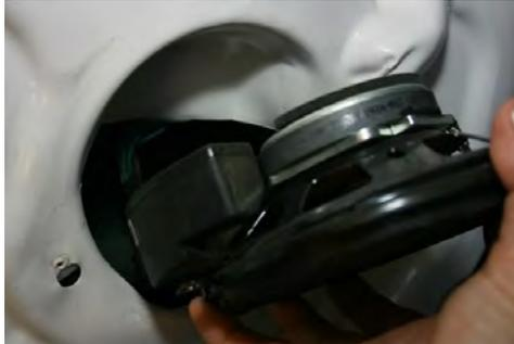
Now the fun begins. After pulling off the fabric dust cover from the front of the speaker, I saw that the ring of foam that holds the speaker cone to the speaker frame had indeed come unglued from the frame. This detached foam, flapping against the frame, was responsible for the rattling, popping, and snapping sounds.
