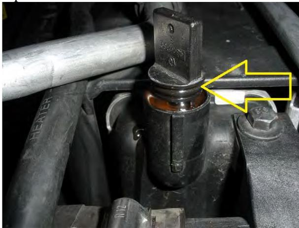
By the way my water pump was just starting to leak out of the weep hole at 101k It could not have made it to 200k I don't think any water pump would make it so plan on doing the water pump and the timing belt. the old belt had one small crack it's hard to see it in the picture but it's there and it had a small amount fibers where the rubber had worn down it did not look new and that small crack could have become a big problem...
