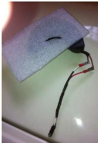
OEM amp with ethafoam pad mounted and wiring pigtail installed.
