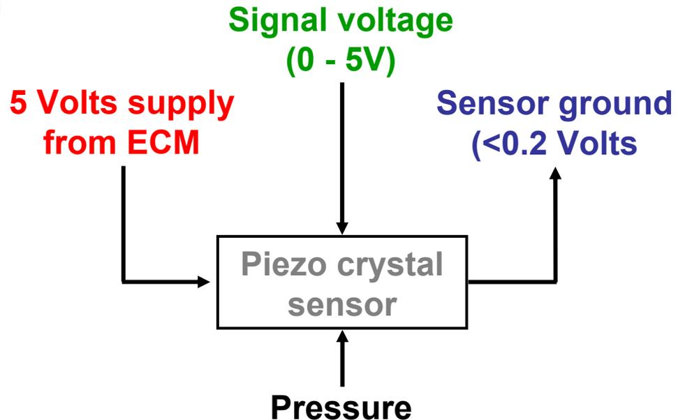
The engine ECM applies a stabilized 5 Volts supply to the signal wire of the fuel pressure sensor.....
