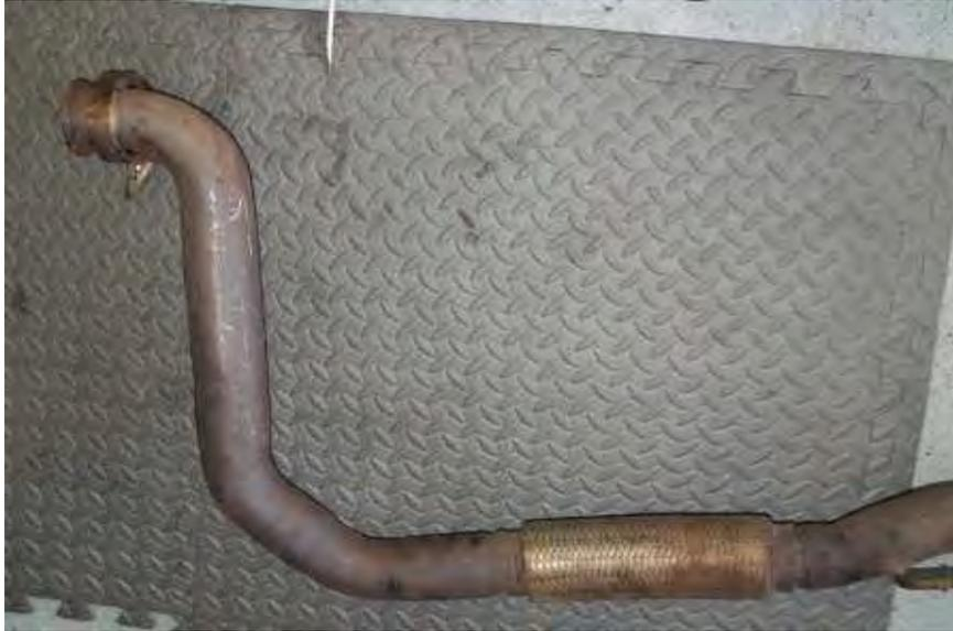
17. Mark the exhaust pipe 3 inches in front of the protruding portion of the flex joint, this is where the pipe needs to be cut to remove the front portion of the downpipe. De-burr the pipe after cutting and sand the last 3 inches of the cut pipe to ensure a clean welding surface.
