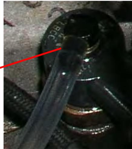
There should **not** normally be any fuel collected in receptacles during engine cranking.
