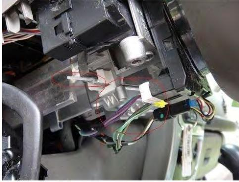
Ignition switch removed showing left end of actuator pin
