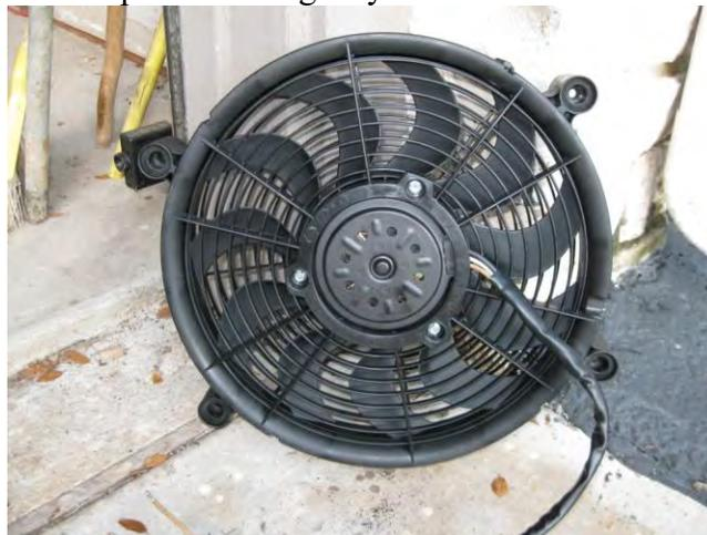
The fan would fit inside the OEM fan shroud if I removed most of the Lugs from the Haden shroud and cut out the grill portion of the OEM shroud.
