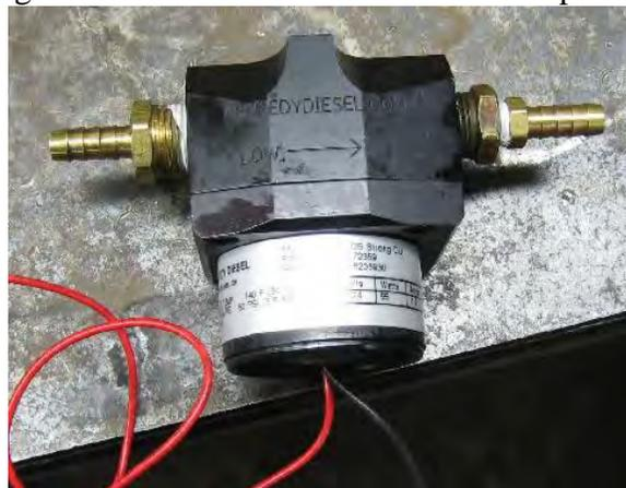
I ordered the Kennedy lift pump from [Kennedy Diesel](#) (the fittings weren't included). It is a centrifugal type which won't cause a restriction if it fails.
