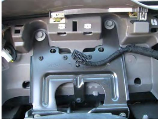
(5) Remove the instrument cluster from the instrument panel.
