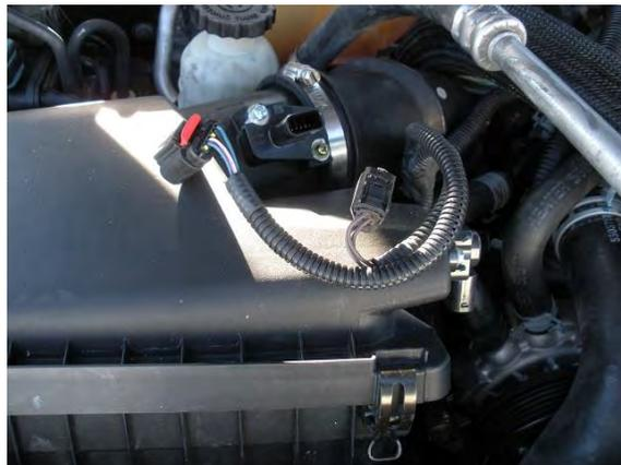
Disconnect the air hose and pull up on the air box remove it...
