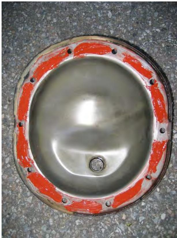
So here came the problem. The gasket kept moving around when I was trying to bolt the cover back on so I decided to use some old RTV i had laying around to hold it in place.
