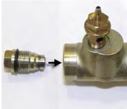
A mechanical pressure limiter valve is fitted to some systems. It is located at the end of the fuel rail.
