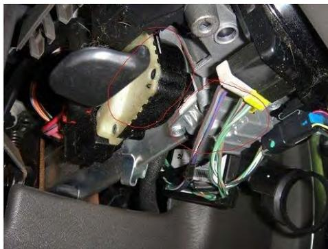
Ignition switch is white/black thing to right of steering wheel tilt release lever handle.
