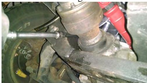
I loosened up both sides while under the car, but only remove one (this case driver side) nut, since we need the passenger side mount secured to the engine and chassis till we change the driver side, to make sure the engine will not move left or right while mounts are removed.
