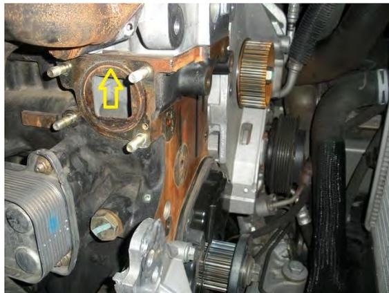
This hose is under the water pump and would be very hard to replace without taking out the pump so even if you don't replace all the hoses you should get this one is a cheap hose and it would be a lot of work to replace it later.
