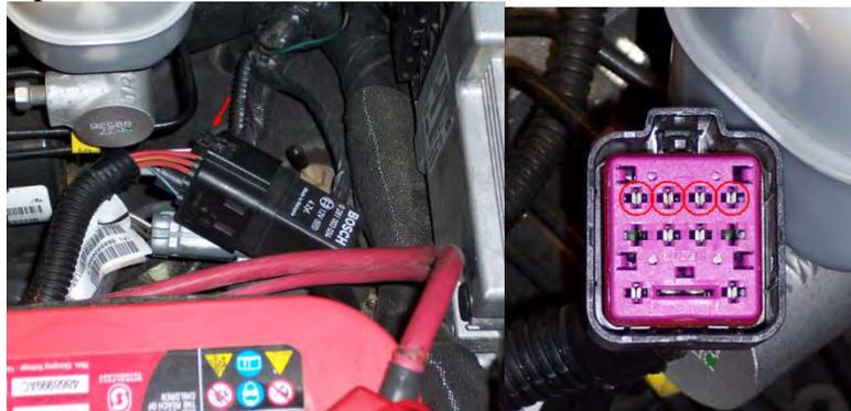
Connect one lead of the ohm meter to the negative battery terminal and measure at the indicated terminals. Unless the wiring harness is on backwards (can happen), the glow plugs should be 4-3-2-1 (left to right).
