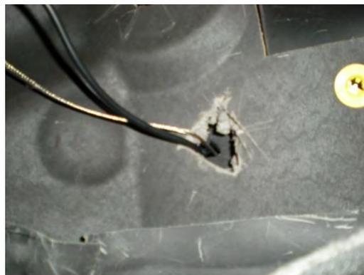
At this point I also ran the 'constant power' lead through the grommet and out to the battery posts (left hand side of the relay box is a good place to attach it with an inline fuse holder). The constant power lead is necessary to maintain the peak reading memory in these gauges - I assume.
