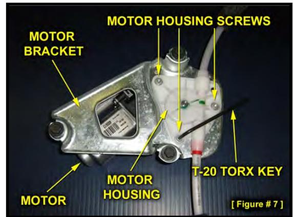
Use the Torx tool provided in this kit (or a T-20 Torx driver) to remove the three motor housing screws (*Figure 7*) then set the motor and the motor bracket aside.
