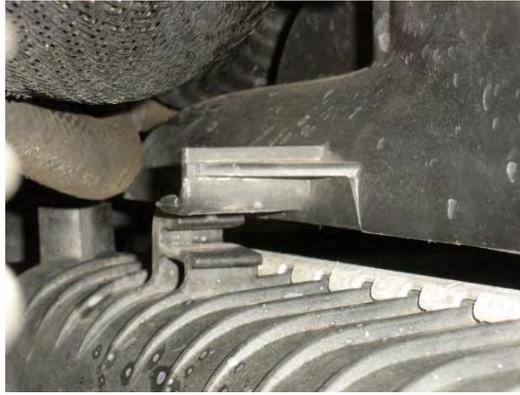
Remove the fan and shroud carefully don't drag the fan against the radiator.
