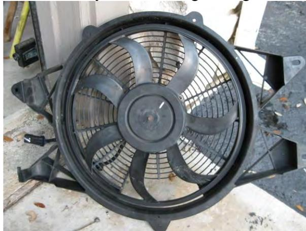
Now from the opposite side (front of vehicle side - fan rotates counterclockwise)
