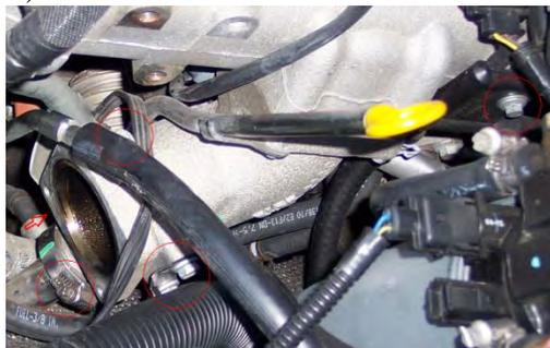
Loosen the clamp (7mm) on the EGR pipe enough to slide it off of the flange and down the pipe. Remove the pair of 10mm bolts shown holding an electrical cable bracket. Remove the (long) 8mm bolt at the far right.
