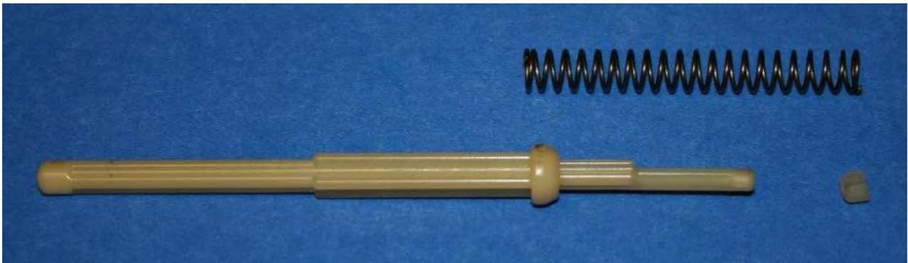
Of course you cannot buy this 50c part so you either have to improvise your own fix or drop \$\$\$ on the entire shifter mechanism. Here is my solution machined from brass so it should last the life of the vehicle
