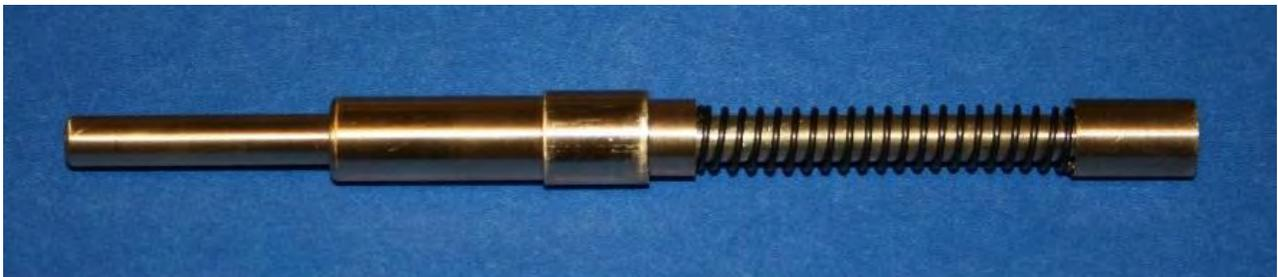
Of course, you could replace with a solid rod. Maybe a chopstick cut to the correct length and do away with the spring altogether. The spring simply allows the rod to "give" if you push the release button on the shifter lever
