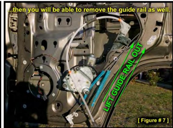
At this point, you can lift the guide rail out as well. The next step is to disassemble the regulator.
