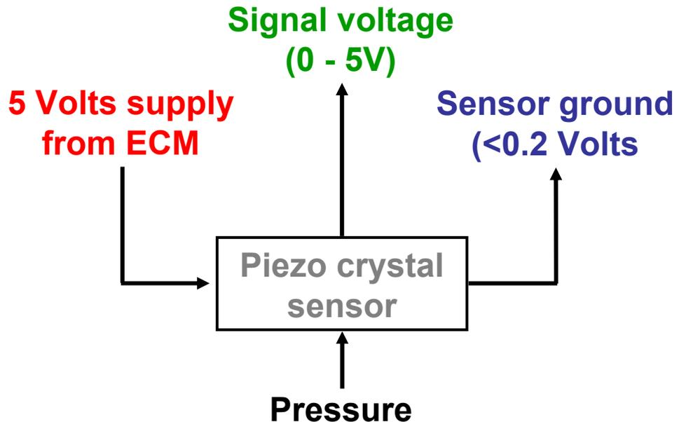
Typical signal voltages from rail pressure sensor:
