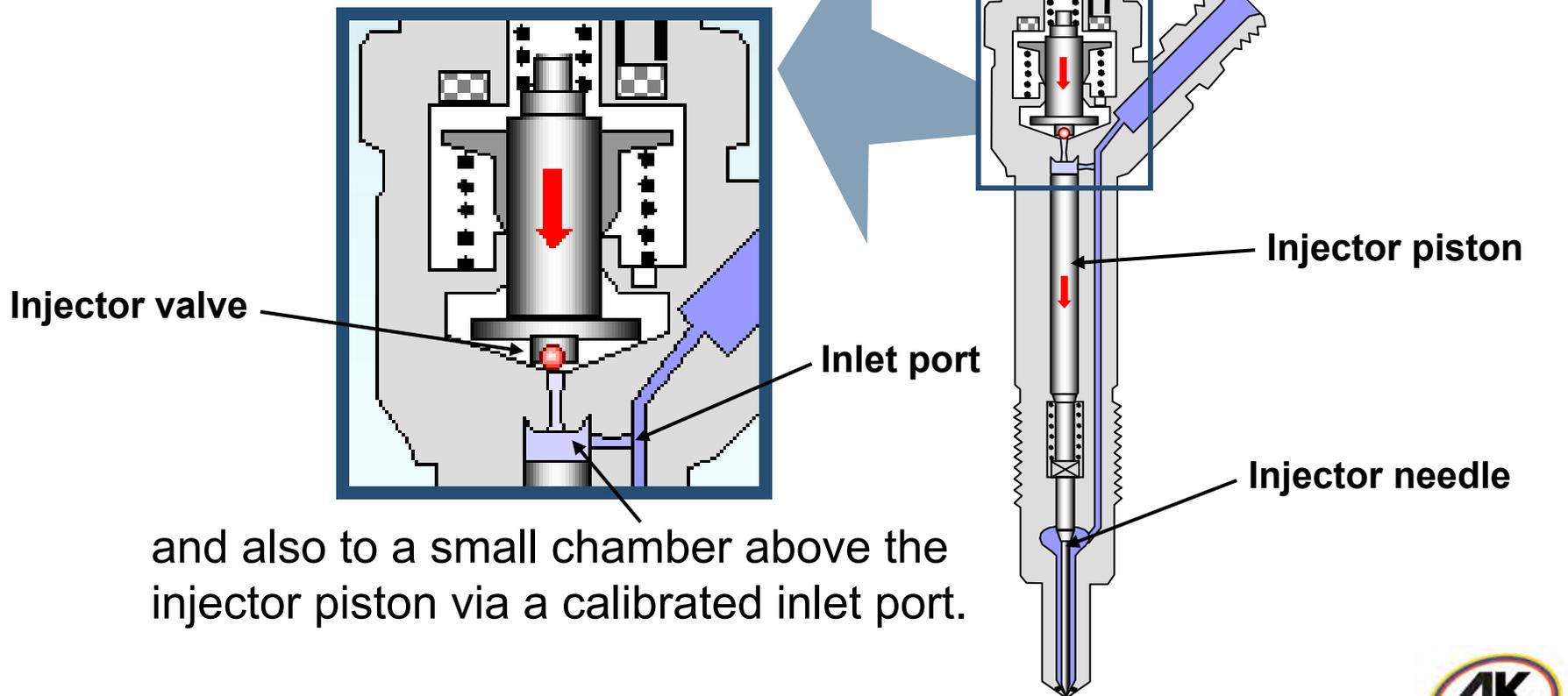
and also to a small chamber above the injector piston via a calibrated inlet port.
