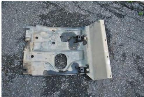
engine skid with out the plastic cover in it. In case anyone is wondering what that oil is from, its from some good ol PB blaster
