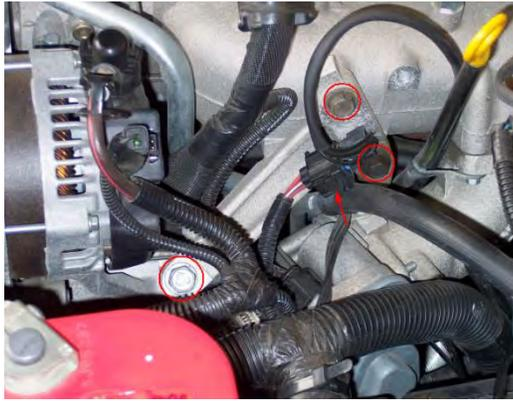
To gain access to #2 glow plug, remove the alternator rear "T" bracket (13mm and 15mm). Squeeze the black tab (red arrow) and unplug the harness connector to the glow plugs. Flip the bracket out of the way.
