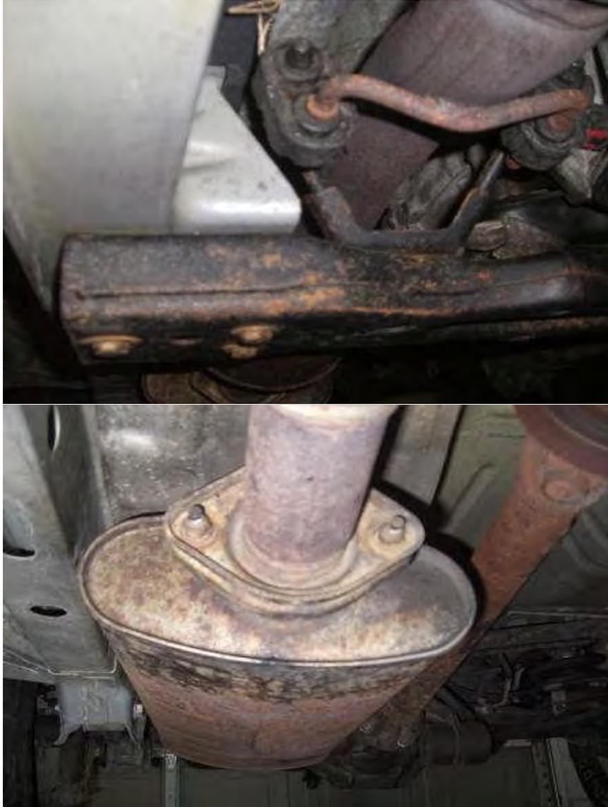
14. Use a pry bar or long screwdriver to pry the exhaust hangers free from the isolators.
