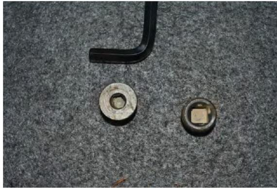
As you can see, the drain plug uses an allen wrench (10mm) but the filler uses some thing else that I didn't have soo....
