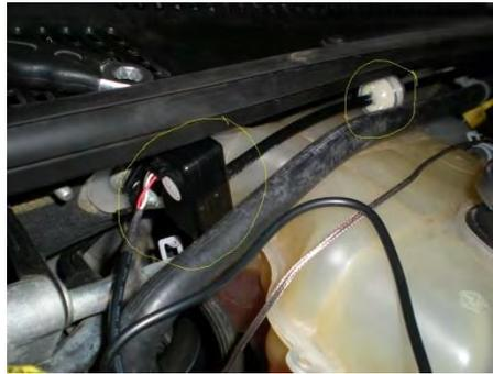
Next fitting the EGT probe (drill and tap the exhaust manifold) and consult Patarcy's post on how to do this. I opted to drill it without the engine running and used the shop vac to pull stuff away from the hole, then used a magnetic screw driver to fish out the tiny bits that might have fallen into the hole.
