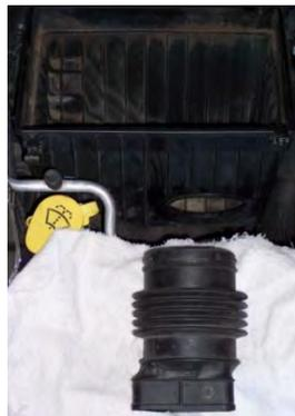
Remove the intake duct from the airbox. You may need to spin it 90°.
