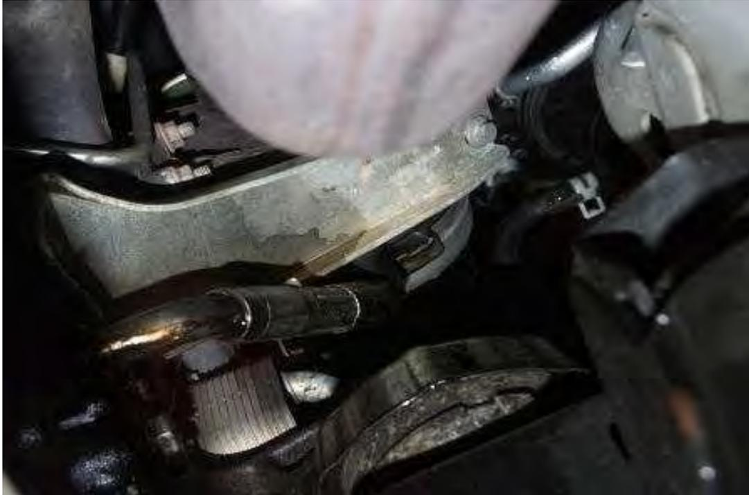
20. On the topside, remove the bolt holding the turbo oil supply to the turbo using a 14mm socket. Make sure to keep the two copper washers that seal the banjo fitting (top and bottom).
