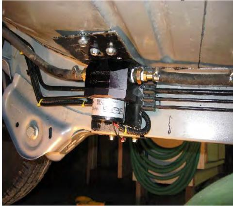
Here is the installed pump. I spliced into the 3/8" metal fuel line and used 3/8" fuel hose to connect the pump. I wanted to make the mounting bracket a little more protective but given the flow direction and mounting bolt configuration my choices were limited. The mount is rock-solid.
