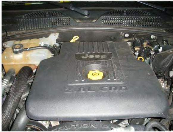
Pull straight up on the engine cover and remove it...
