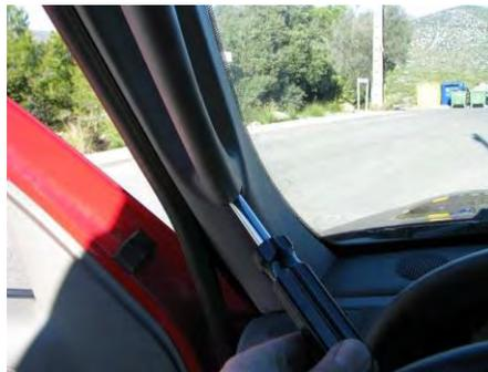
(2) Remove the instrument panel top cover. (lift the left side only to access cluster screw)
