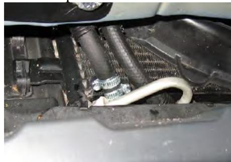
The new cooler outlet is connected to the factory line. I used plenty of ziploom to protect the lines.
