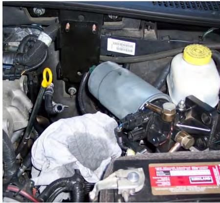
To gain access to #4 glow plug, remove the hose on the top left of the fuel filter and the two 13mm nuts holding the fuel filter to the firewall mount. Set the filter to the side.
