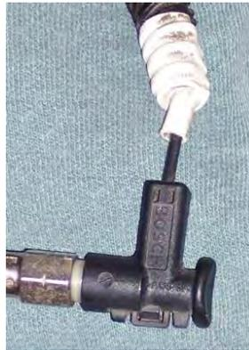
Remove the glow plug connectors. They are tucked under on the side of the engine. This plug wire has a white band indicating that it should be on the #1 glow plug (closest to the alternator).
