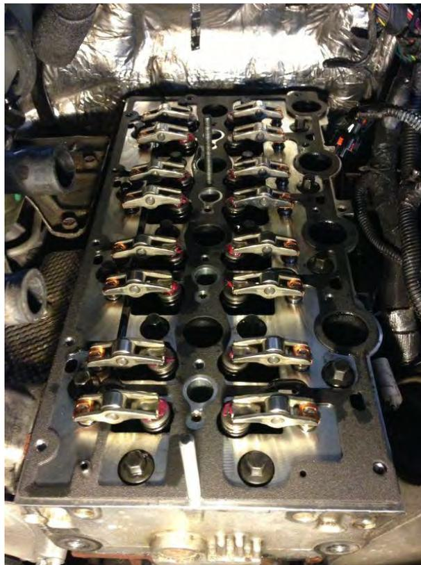
To move away the wiring from the top of the head (visible in one of my pics), remove the wires from the plastic harness, use some cable ties to group them together, then tie them with an electric wire on one end, and the
