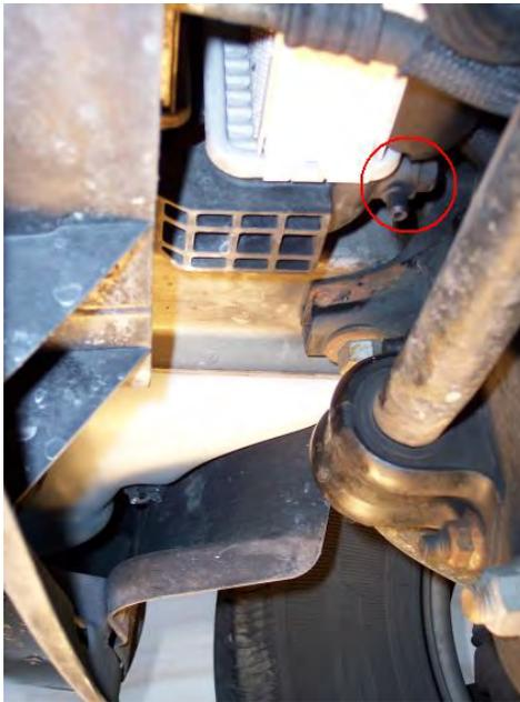
The engine should be cold for this procedure. Turn the cabin heat on to full (engine not running). Disconnect the battery. Attach a 5/16 inch hose to the radiator drain cock. It is on the inside, passenger side, lower corner. Feed the hose into a clean bucket; we will save the coolant.
