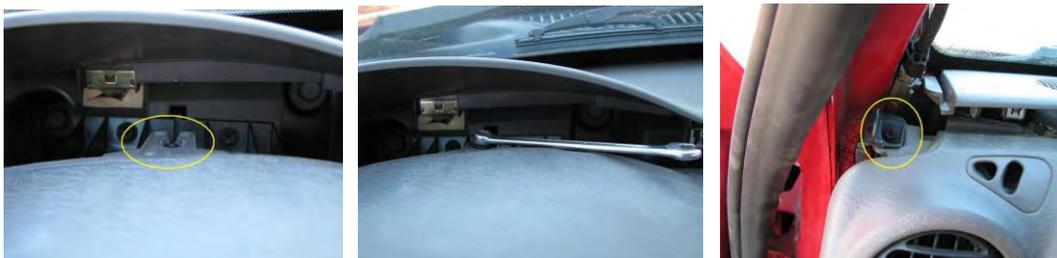
There is a piece of plastic covering this hole for some reason, take off fuse box lid and door seal to take it out / fit it back the right way.
