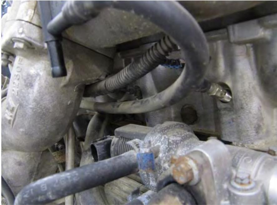
Passenger side view with heat shields in place. Turbo to left with oil return line running down from it to the block and rectangular oil cooler slightly below and to the right.
