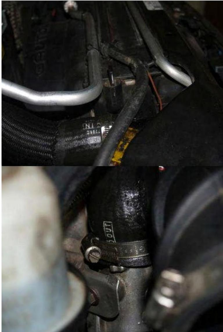
4. Loosen clean air intake duct from air box and then remove air box assembly after disconnecting the mass air and air box pressure sensors.
