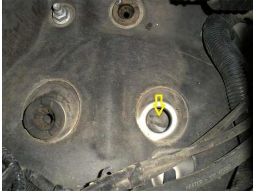
some grease on the grommets will make it easier to reinstall the air box...
