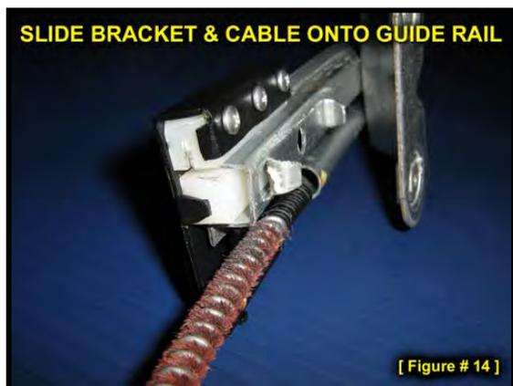
Slide the broken plastic bracket off the guide rail and install the new one as shown in Figure 14. The cable rides in the round channel, the nylon block in the middle of the bracket rides in the square channel and the nylon slot rides on the edge of the guide rail.
