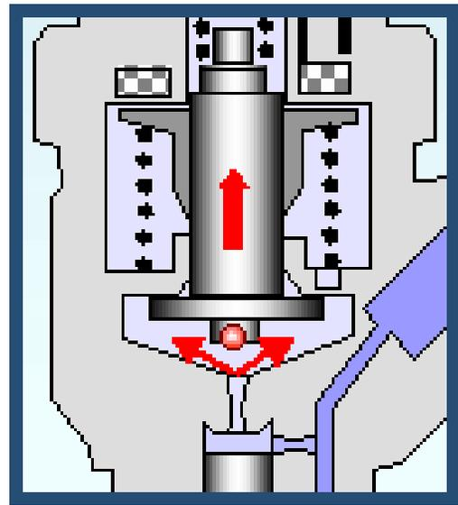
Fuel pressure below the injector needle lifts the needle.
