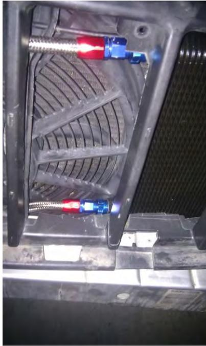
See how the plastic is trimmed to allow the cooler to pass behind
