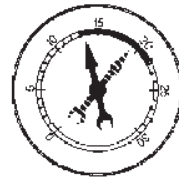
WORN VALVE GUIDES (STEADIES AS ENGINE SPEED INCREASES)
