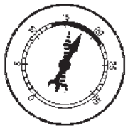
POOR VALVE SEATING AT IDLE
