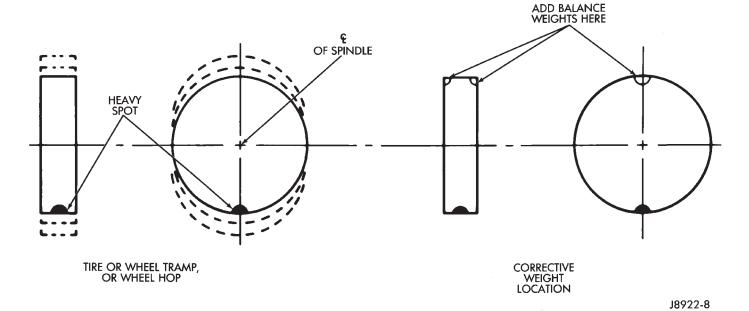
Fig. 6 Static Unbalance & Balance
