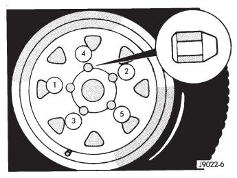
Fig. 5 Lug Nut Tightening Pattern
