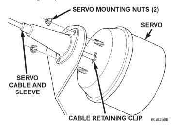
Fig. 4 Servo Cable Clip Remove/Install—Typical
