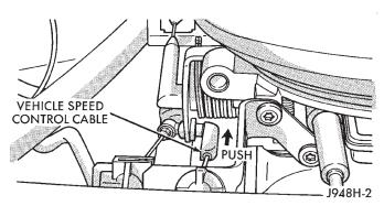
Fig. 7 Cable at Bell Crank—5.2L/5.9L V-8 Engines
