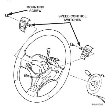
Fig. 5 Speed Control Switches
