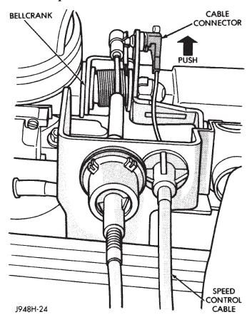
Fig. 6 Cable at Bell Crank—4.0L Engine
