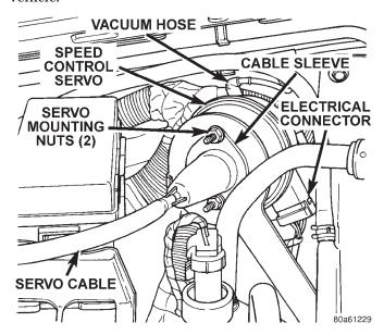
Fig. 3 Speed Control Servo Location
